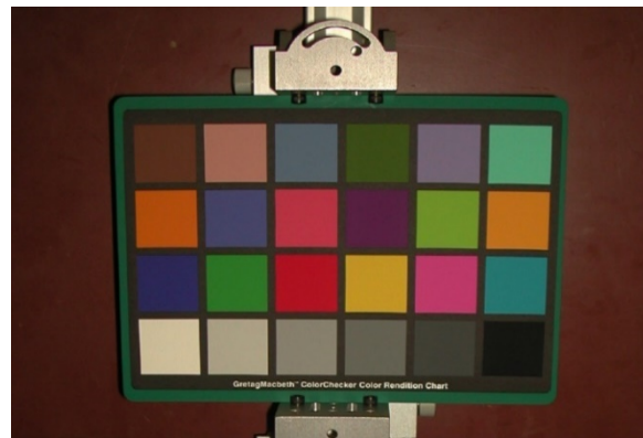
Testing the accuracy of distance determination using planar targets
